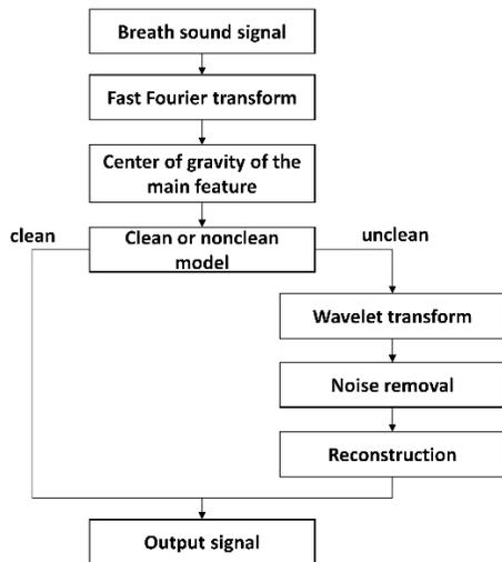
Figure 1. Flowchart of signal processing.
