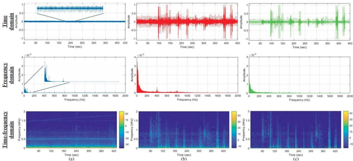
Figure 2. Breathing sounds: (a) clean, (b) nonclean and (c) denoised. Top row: time domain, middle row: frequency domain, and bottom row: time-frequency domain.
